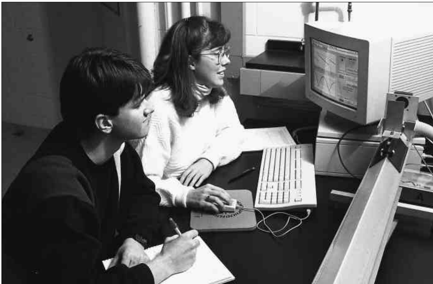
Aaron Hexamer and Sarah Bekofske study the motion of a glider floating on an inclined air track with a sonar transducer in the Physics 152 Laboratory. Photo credit – CIS Photographic Services, Purdue University.
