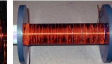
1a) Begin winding the coil by first passing the end of the wire through a mounting hole. Here, the first 3 turns are shown. Notice how tightly the coil is wound.
