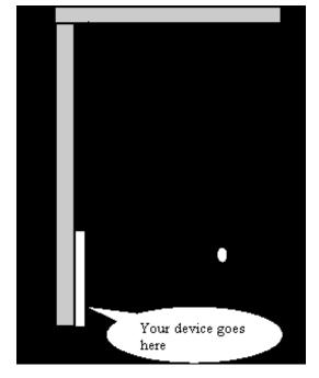
The thickness of your egg catcher will be measured from the board to the thickest point of your device.
