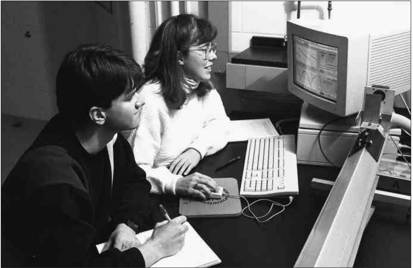
Aaron Hexamer and Sarah Bekofske study the motion of a glider floating on an inclined air track with a sonar transducer in the Physics 152 Laboratory. Photo credit – CIS Photographic Services, Purdue University.
