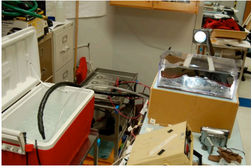
Setup prepared for operation. Note the ice bath to the left, cloud chamber to the right, and overhead light source behind the chamber.
