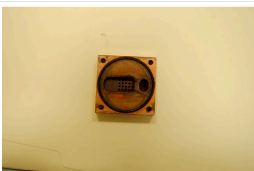
Inside of the copper water jacket. This one was removed and taken apart because of a freeze failure.
