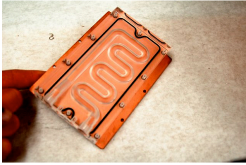
Opposite side of the hard drive cooler.
