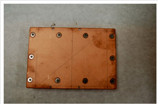
Scribe marks on hard drive cooler for placement of two thermoelectric units. This type arrangement found to be ineffectual because the large surface area leaks heat back to the aluminum plate.
