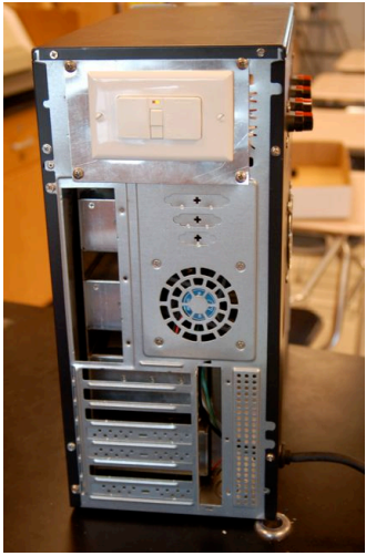
GFCI switch turns on the four internal power supplies.
