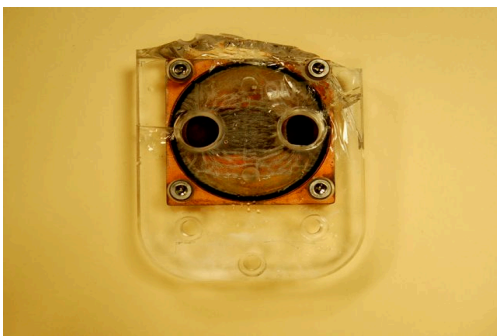
Working at near freezing temperature can be hazardous. The plastic was replaced with machined aluminum blocks for all four heat exchangers.
