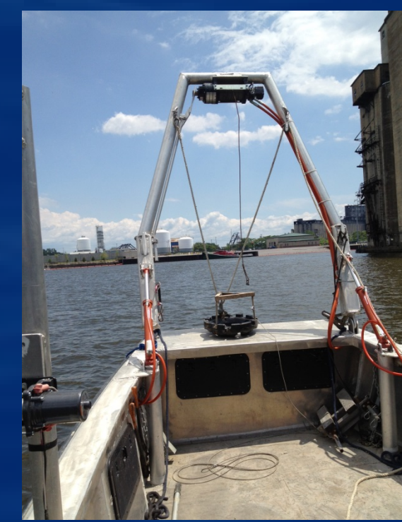
Block and tackle style deployment of temperature sensor
