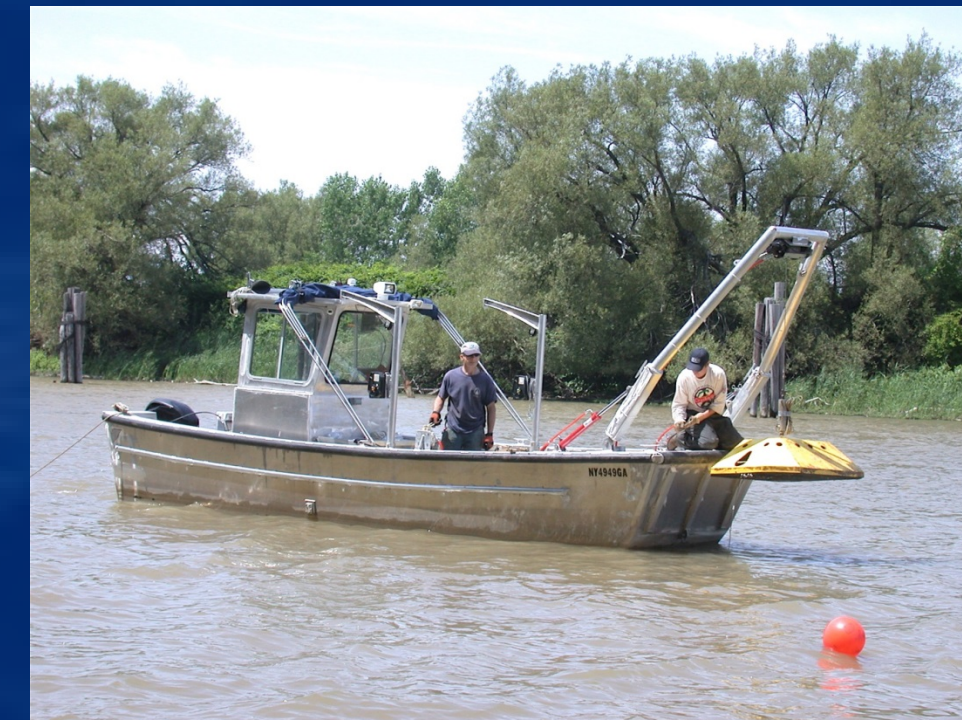
Deployment of a vertical acoustic doppler profiler
