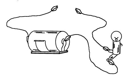
Use the materials given to make an electric tester. Use the tester to check if an electric current flows between all the various pairs of terminals (A to F) on the circuit board.
