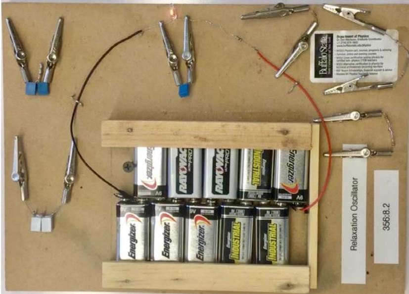
Figure 2: Our RC Neon bulb “blinky” circuit with additional clip-in Capacitors and Resistors for experimentation
