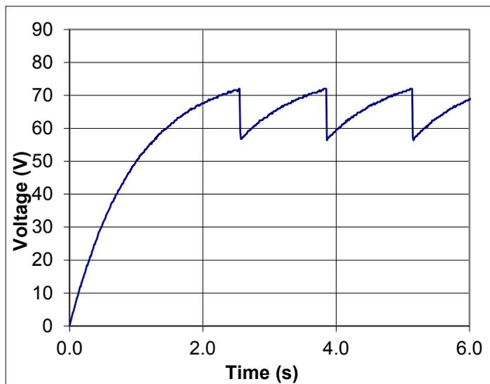
Figure 5: Capacitor potential  $V_c$  vs  $t$  for  $1\text{M}\Omega$  &  $1\mu\text{F}$  (Digital oscilloscope data by S. Wilser)
