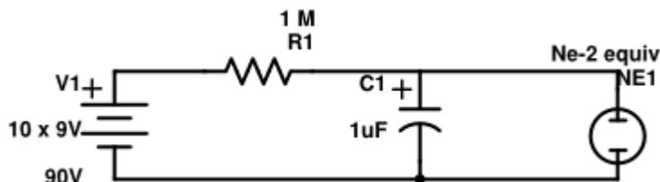
Figure 4: The Relaxation Oscillator (Neon blinky) circuit diagram
