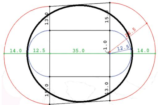
*Figure 1.* This image shows the dimensions of the Regulation track of the Women’s Flat Track Roller Derby Association ([wtdfa.com](http://wtdfa.com)), all dimensions are in feet. The thick black line shows a circular path skated for speed measurements. Retrieved from [rules.wtdfa.com/](http://rules.wtdfa.com/) with author modifications.
