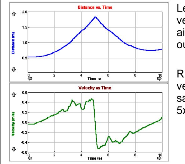
Left: distance and velocity data of an air track glider without a reflector.
