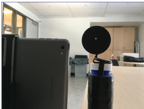
Fig. 8. The pinhole image size is now approximately equal to the point source, indicating the camera lens is located at the focal plane.
