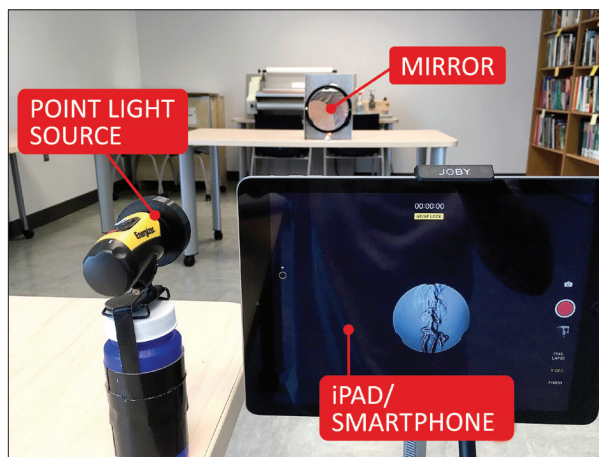
Fig. 6. Setup using LED flashlight, iPad mounted to a tripod, and a parabolic mirror.
