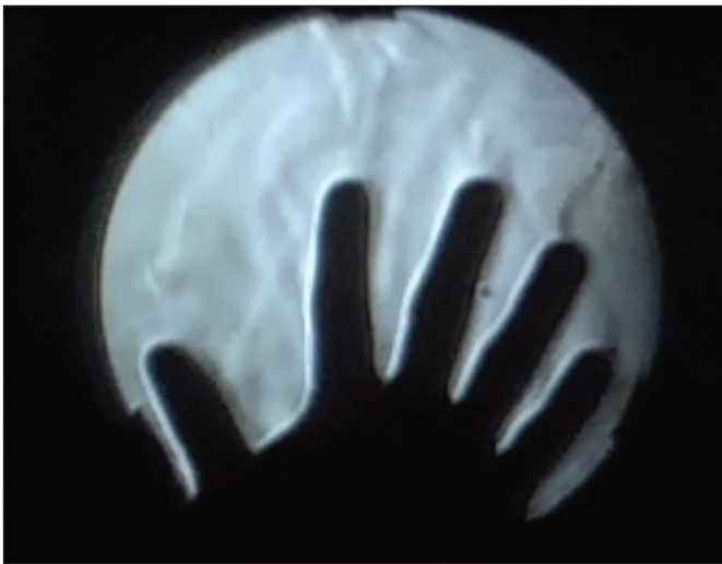
Fig. 12. Rising convected air shows heat exchange between a warm hand and the surrounding air.
