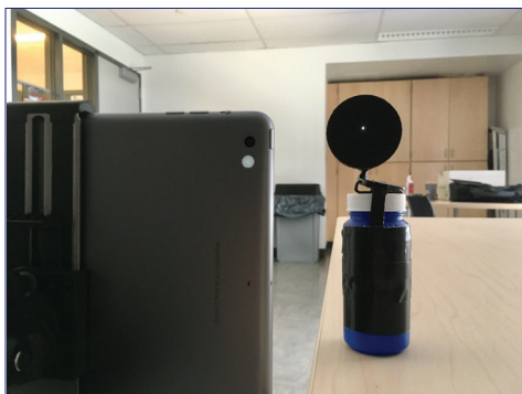
Fig. 7. The large pinhole image size projected onto the back of the iPad below the camera indicates the iPad camera lens is not located at the focal plane.
