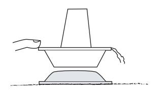
e.) Pull the electrophorus away from the plate. The electrophorous now has a net charge. Draw the charge on the pie tin.
